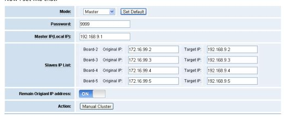
At first, I set the Master IP(Local IP) is 192.168.9.1,I give another IP to the first board(172.16.99.1), now the first Board have 3 IP address, one is 172.16.99.1, one is 192.168.99.1(Reserved IP address) and the other is 192.168.9.1.
