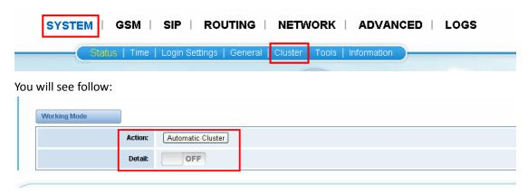
Now OpenVox GSM Gateway can support 2 ways to configure the cluster. One is manual, the other is Automatic. At first, we cluster manual.
