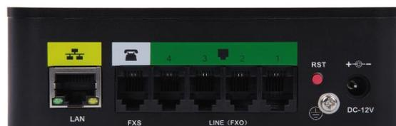
Figure 1-2 UC300-A41EM1 back panel
