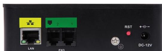
Figure 1-2 UC300-A11EM1 back panel
