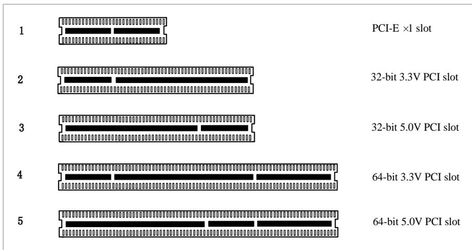
Figure3 PCI-E and PCI slots
