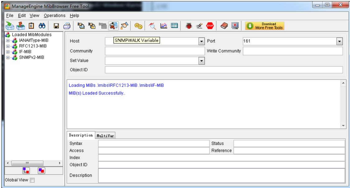
And the field of **Host**, **Port** and **Community** are filled with **172.16.100.223**, **161** and **public** respectively. Object ID is the node of SNMP MIBs, e.g. “.1.3.6.1.2.1.1.6.0” is system location and “.1.3.6.1.2.1.1.1.0” is system description.
