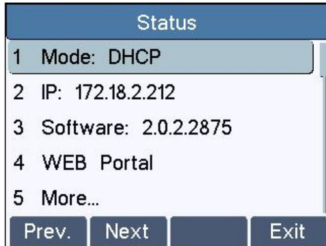
Figure 7 - Check the Device's IP Address
