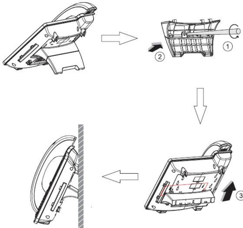
Figure 2 - Wall-mount Installation
